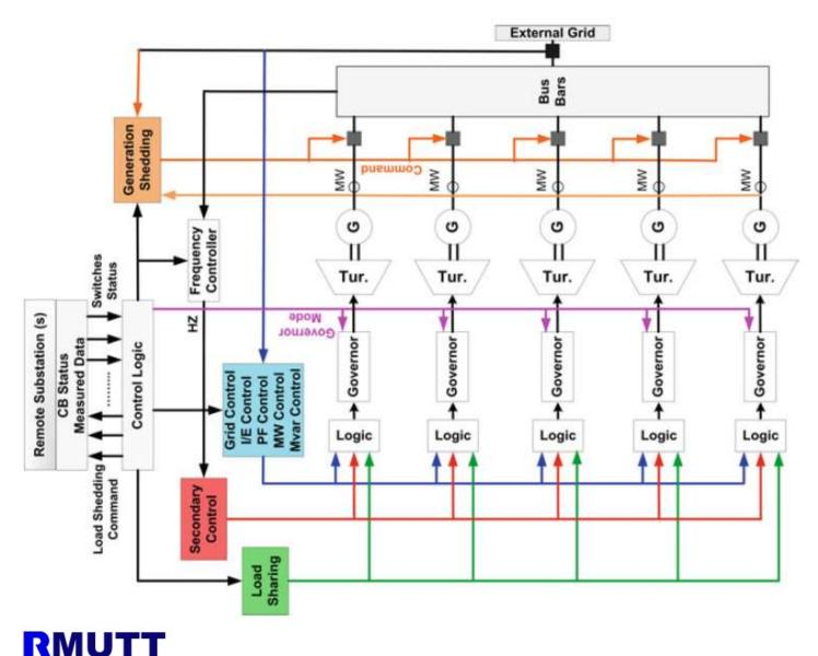
Example: Overall schematic of smart power management system controllers
